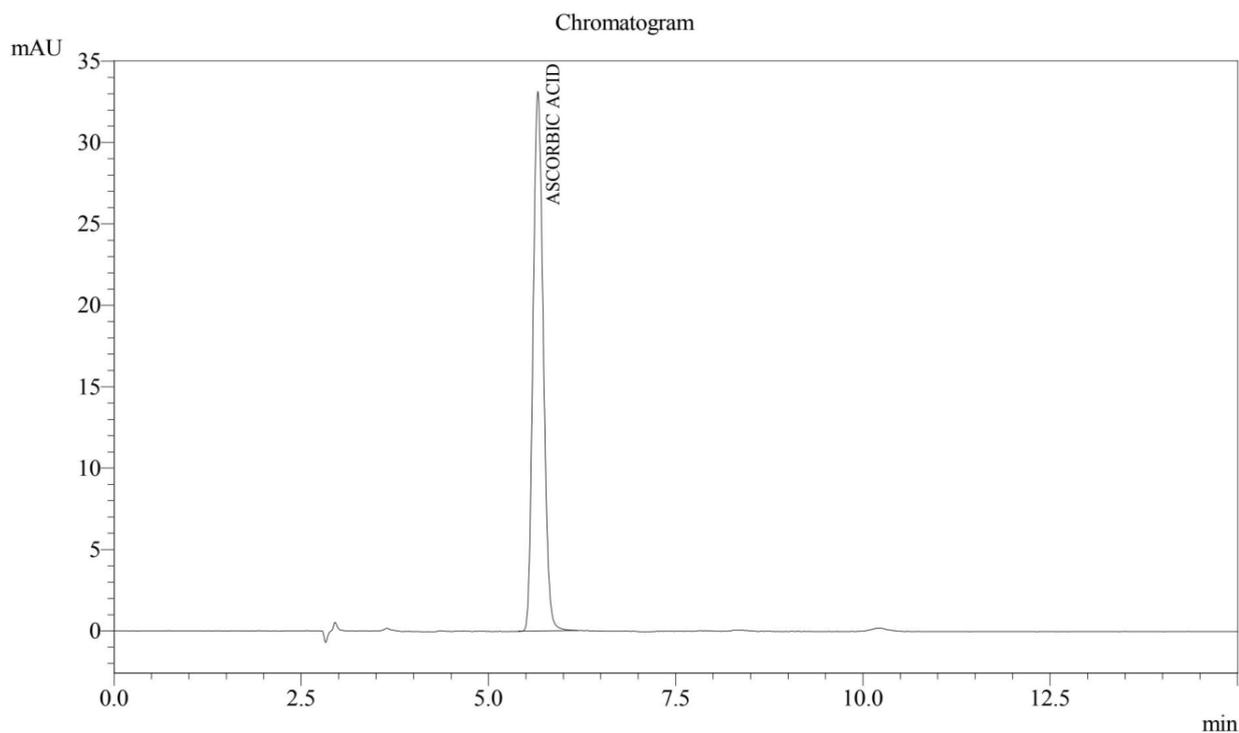
**Fig 1: The HPLC Chromatogram of Standard Ascorbic Acid.**
